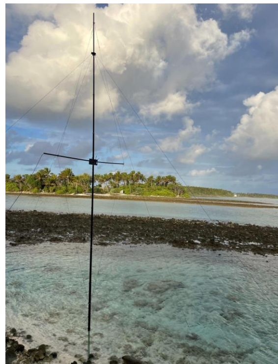
Zeke VDA antenna for 15m Band placed within the ocean on Majuro Atoll.
